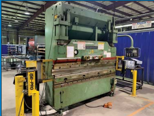
90 Ton x 8' Cincinnati Autoshape Model 90AS CNC Press Brake
