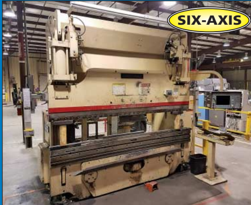
90 Ton x 8' Cincinnati Autoform Model 90AF CNC Press Brake w/ Crowning
